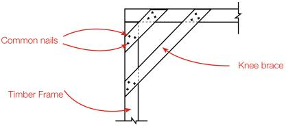
Possible timber knee bracing detail: by having dual braces the joint
